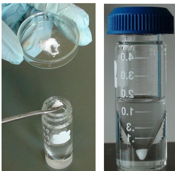
Figure 12. Drying with anhydrous calcium chloride.
